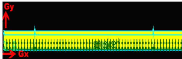
**FIGURE 4. GEOMETRIC MODEL FOR THE TUBE WITH MESH INSERT (10MM MESH DIAMETER AND 2.5MM PITCH)**
