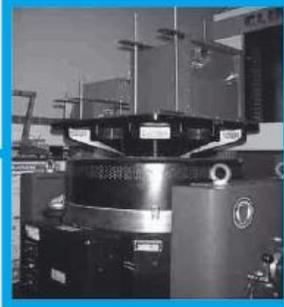
The laboratory is part of the Department of Mechanics of the Royal Military Academy. LDMS is able to perform vibration testing in order to simulate the environmental, mechanical conditions that act on a product or structures. The laboratory can perform a research of resonance frequencies, a sine dwell, a sine sweep, random vibrations and shock tests in accordance with several standards, such as MIL-STD-810, IEC 255-21-2, IEC 60068-2 series,...
